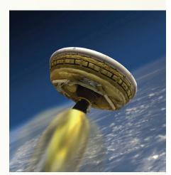
Kauai. At 34 miles up, Earth's atmosphere resembles Mars'. A massive balloon and then a rocket motor will elevate the LDSD to its high point, where it will then begin its plunge back to Earth at a speed of roughly 3,000 mph. Once that speed is reached, the inflatable bladder will fill with gas and expand to nearly 20 feet in diameter, which will cut the LDSD's descent speed by half, enabling a massive parachute (110 feet across) to unfurl and gently guide it to the surface—theoretically.
